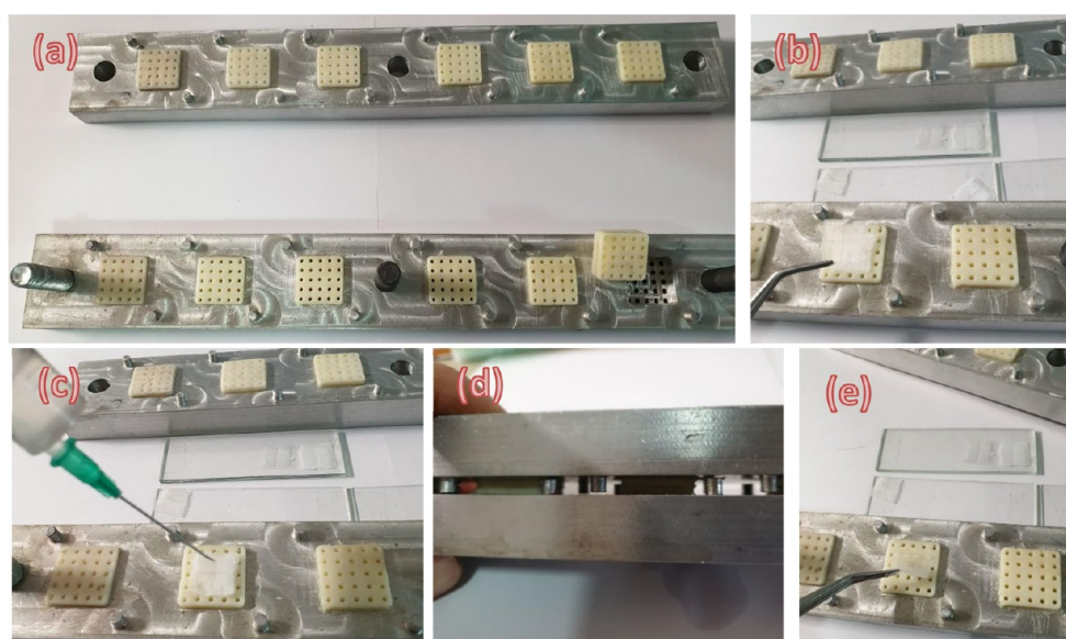
Figure 12. (a) Aluminum sintering fixture with six sintering cavities. (b) Placing layer by layer of scaffold and aligning them with each other. (c) Adding some methanol to fix the layers relatively. (d) Sintering the fixture in closed position. (e) Peeling off the solidified layer.
